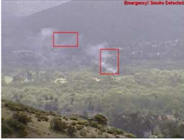
Figure 4. A snapshot from an independent test of the system by the Regional Technology Clearing House of San Diego State University in California in April 2009. The system successfully detected the test fire and did not produce any false alarms. The detected smoke regions are marked with bounding rectangles.
